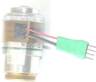
2. Wrap the heater around the objective, and mark the point where the end of the heater with Velcro already attached will be placed. Adhere a piece of Velcro over the mark. It is recommended to put an excess of Velcro so it overlaps some surface of the objective for extra stability (some Velcro can be cut). Secure the end of the heater inside the Velcro piece. The end already has Velcro attached.
