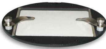
**Uniformly heated glass plate for stereo microscopes, upright microscopes, and long-distance objectives of inverted microscopes, TC-HP75x65** Large 75x65mm optical clearance allows you to heat your samples on 80x70mm glass surface. The heated glass plate provides thin profile and uniformly heated surface. Built-in temperature sensor. Flat glass top surface is flashed with the microscope adapter. Can be used to heat plates, flasks, slides and petri dishes.
