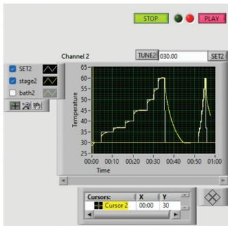
Below is an illustration of “ramp” protocol recordings to show that the controller will “follow” the ramp well, provided the rate of the ramp is slow enough. The last ramp down was too fast for the controller to “follow”.
