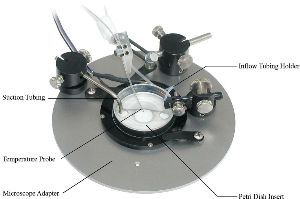
**4b** Another way to achieve the correct temperature around your sample is to switch the feedback of the controller to BATH temperature sensor. This might result to temperature fluctuations, however. NOTE: it is recommended to use feedback from STAGE first, so the controller can be tuned to required temperatures inside the heating element (read about compensating OFFSET/gradient temperature and overheating threshold above and below).
