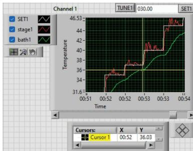
Using an objective heater with oil or water immersion objectives will eliminate this temperature gradient. The second channel of the controller is usually used to regulate the temperature of the objective heater, which has a built-in temperature sensor and does not require too much of fine tuning.
