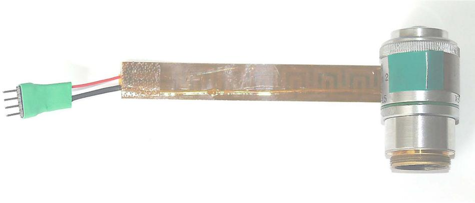
1. Position the heater on the objective closer to the sample plane, the sensor down touching the objective surface, and fix in place using a small piece of electrical tape.
