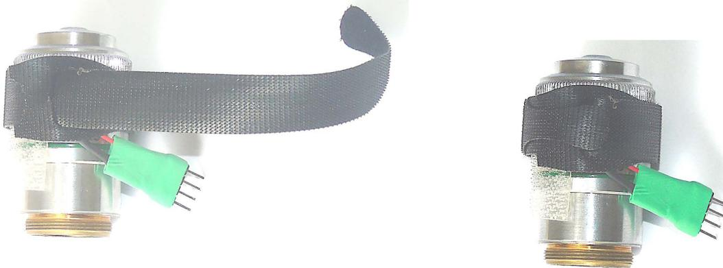
3. Make a loop using black Velcro tape, and tighten it around the heater so the connector is sticking outside from the tape.
