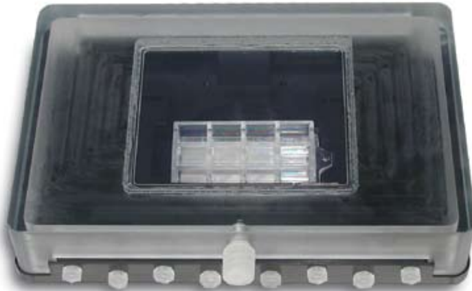
Incubator for motorized stages TC-MI with chambered cover glass inside.
