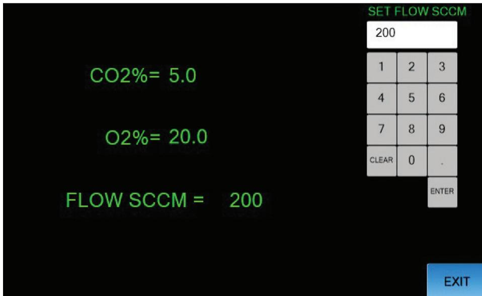
To adjust settings touch SET CO2 button, for example, CLEAR the old settings and ENTER the new one (the same for O2 and FLOW)
