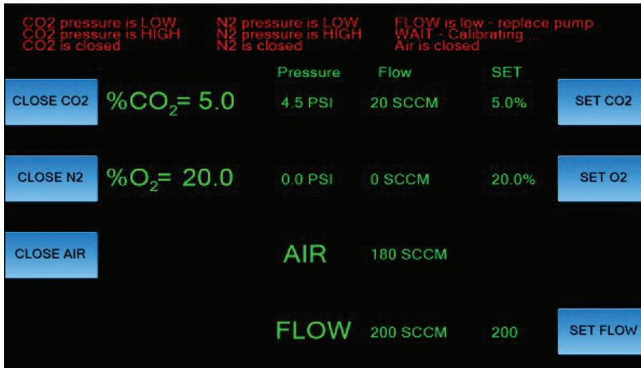
**2** Turn the controller ON. After brief self-calibration procedure, shown as “WAIT - calibrating...”, the display will show concentrations of CO2 and O2 in the output mixture and start making the mixture according to factory settings of 5% CO2 and 20% O2.
