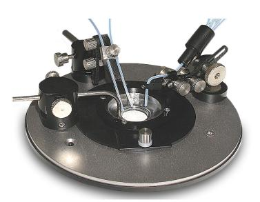
Example of using CSC chamber in a perfusion setup. Magnetic holders are arranged on a microscope adapter MA to provide solution inflow and outflow. 1. Position the bottom part of the 2-parts chamber on a flat surface. Put a cover slip inside the groove in the bottom part. Put the top part inside the bottom part.
