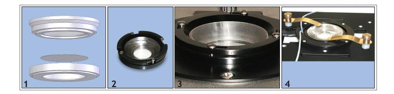
Arrange magnetic holders with inflow manifold and suction tubing around the chamber. While using the cover slips with cultured cells, excess of solution on the cover slip might result in bad seal and cause leakage. Try to leave only a minimum amount of liquid on the cover slip before assembling the chamber.
